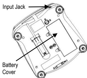
Connect the AC Adapter plug to the input jack.
